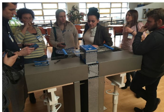
Figure 3: Isothermal load-bearing element supporting a cantilevered balcony floor slab.
