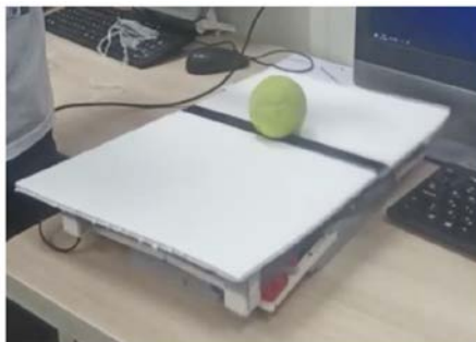
Figure 1: Emulator for a tennis ball contact detection device.
