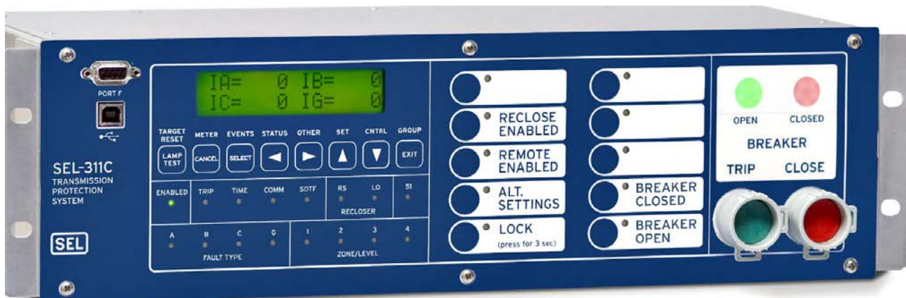
Figure 6: SEL-311C transmission protection system [15].
