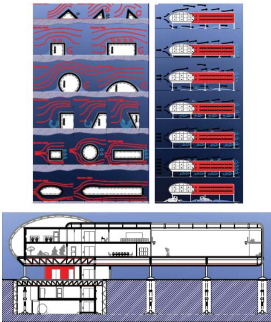
Figure 6: A study of aerodynamics of forms and the resulting solution for an Antarctic energy-effective station (Source: P. Duda and R. Kalinowski, *Diploma design*) [5].
