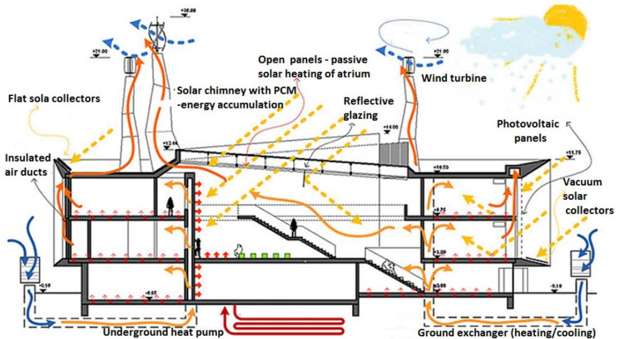
Figure 3: An energy diagram of a building with the close to zero demand for non-renewable primary energy. The building as a system of interrelated solutions. Research and educational complex of the Faculty of Environmental Engineering, Wrocław University of Technology (Source: P. Kuczia, *Educating Buildings*) [4].
