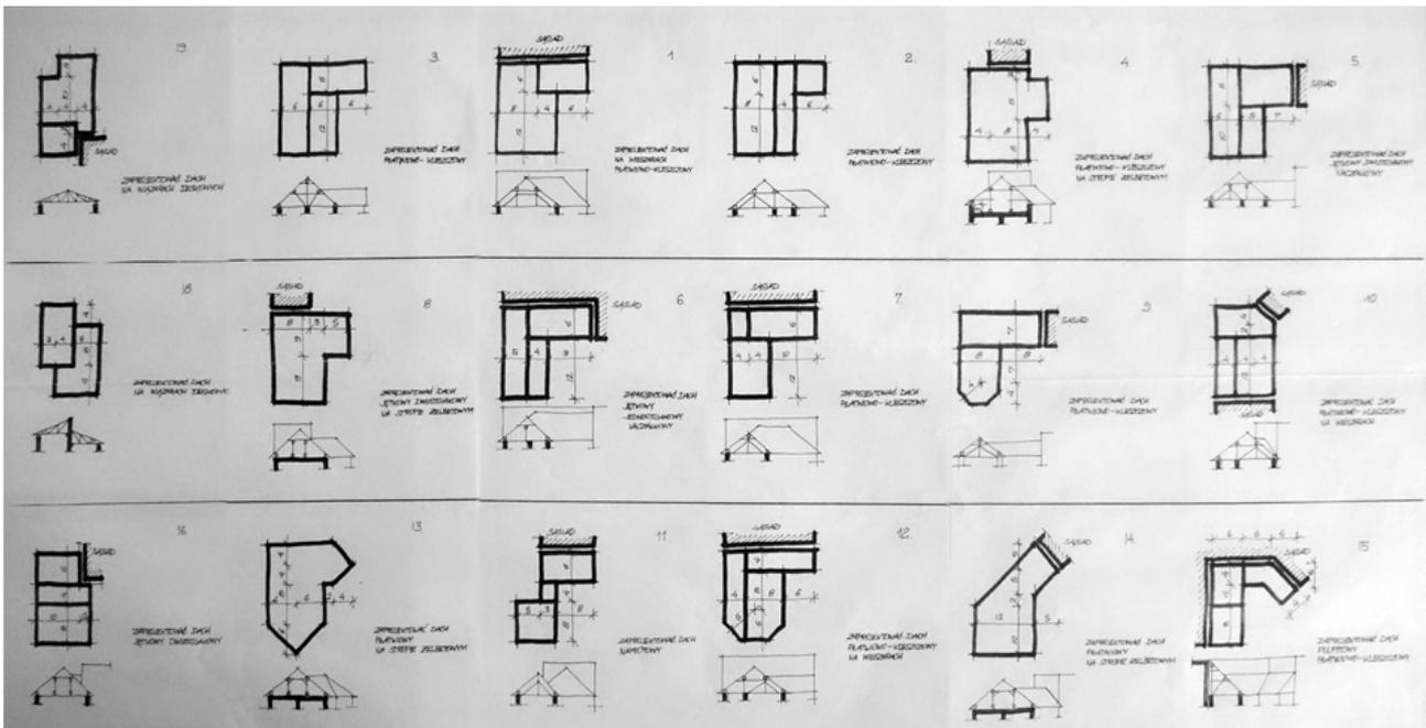
Figure 4: The set of project tasks has multiple variations of shapes and available supports for roof construction, but in fact represents a few traditional solutions for the roof structure. Drawing by R. Marcinkowski.
