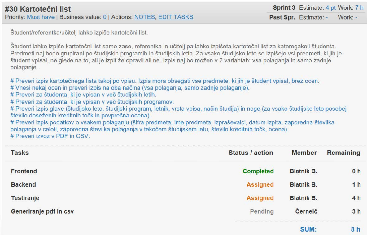
Figure 1: An example of a user story card. The upper part of the figure represents the user story as it is described in the product backlog. The lower part shows the tasks that are added by the team during the sprint planning meeting.
