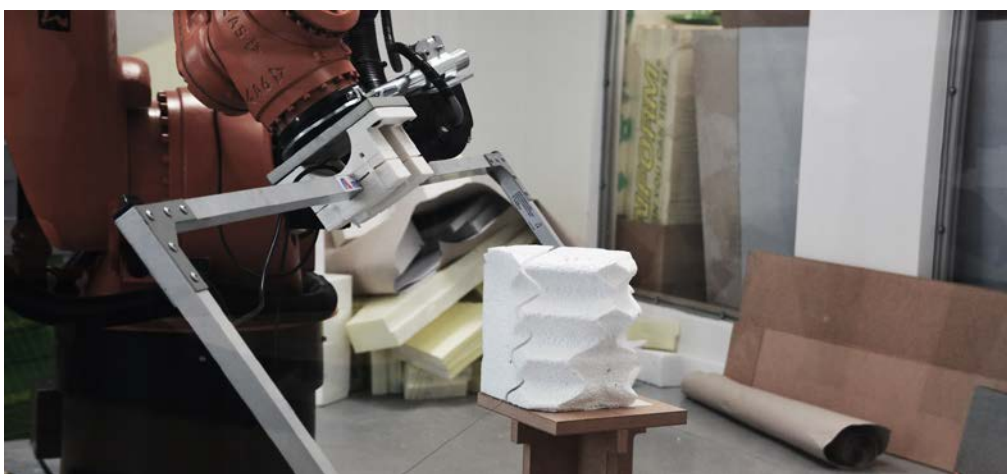
Figure 6: The process of hotwire-cutting with robotic arm.
