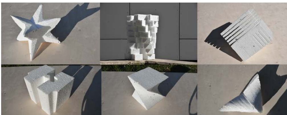
Figure 7: Forms achieved with wire-cutting.
