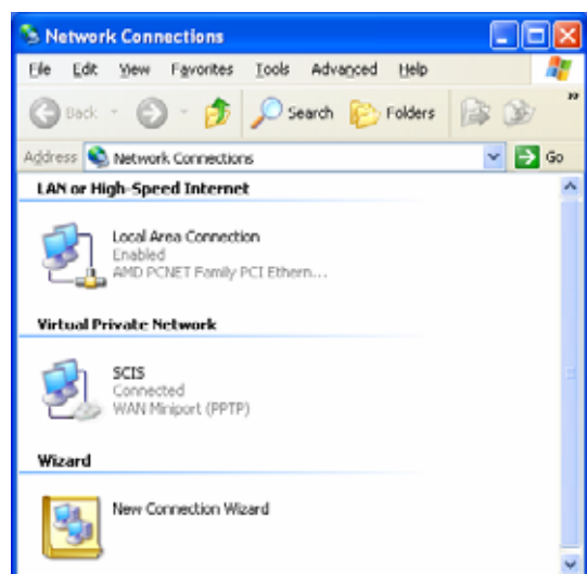
Figure 8: Confirmation at Workstation 2 that a domain user is connected to the Virtual Private Network (VPN).
