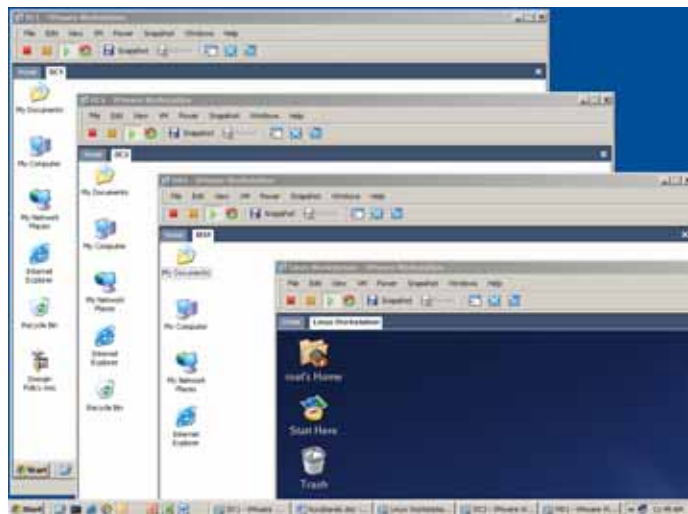
Figure 2: Host computer concurrently running two Windows 2003 domain controllers, a Windows 2003 router and a Linux workstation.
