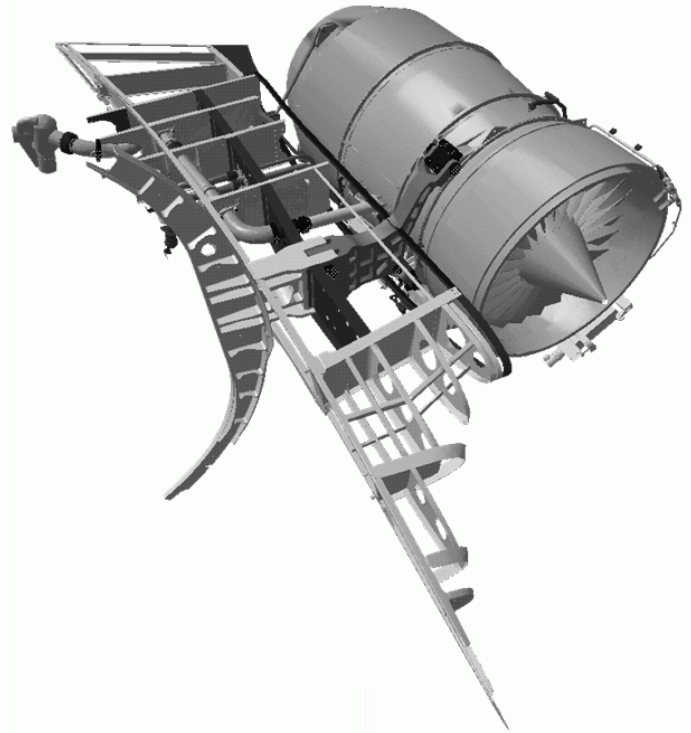
Figure 2: Illustration of the structure and associated systems involved in the CAMAQ pylon retrofit project.
