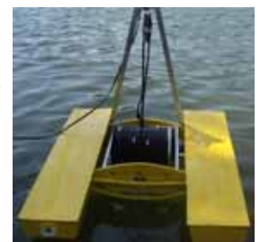
Figure 4: (A) Configuration of the IMAPS for water surface probing; (B) The IMAPS parked in a local lake.
